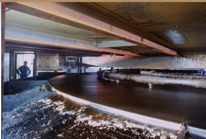
At left, raw bitumen is separated from the sand, water, and clay at the extraction plant to prepare for upgrading. At right, the in-situ process uses steam assisted gravity drainage technology to inject steam into the oil sands and collect the bitumen released by the heat. The recovered bitumen is sent by pipeline to the upgrading facility. The process does not require extraction as separation occurs in the ground.
