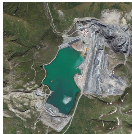
An aerial view of the Red Dog Mine shows the mill facilities, the ore pit and the tailings pond. The Aqqaluk deposit is adjacent to the main pit.
