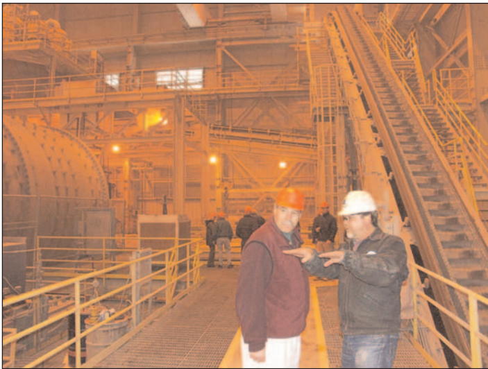
RDC board member Scott Thorson, left, is briefed on mill operations. After the ore is removed from the open pit, it is taken to the "crusher" where large boulders are crushed in seconds. A half-mile conveyor then moves it to the mill for processing.
