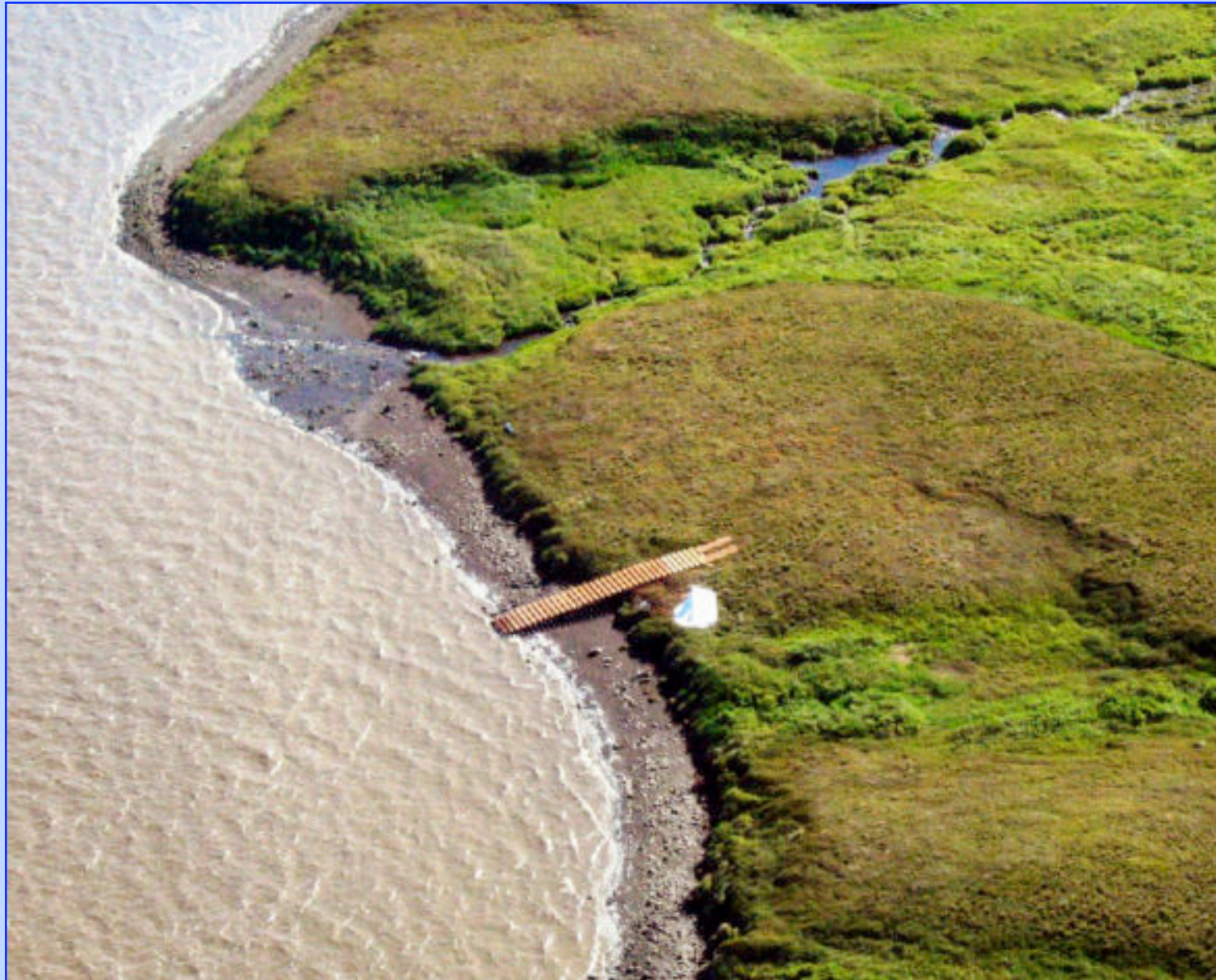
The barge ramp the village built to deliver housing packages to Mertarvik
